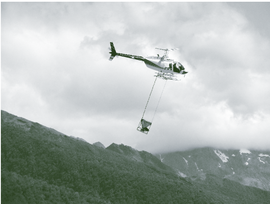
Figure 5.3: Helicopters are used to drop aerial 1080 in rugged areas that are difficult to access. A single helicopter, using a GPS system and mechanised loading, can cover thousands of hectares in one day and control possums, rats and stoats in the same operation.
